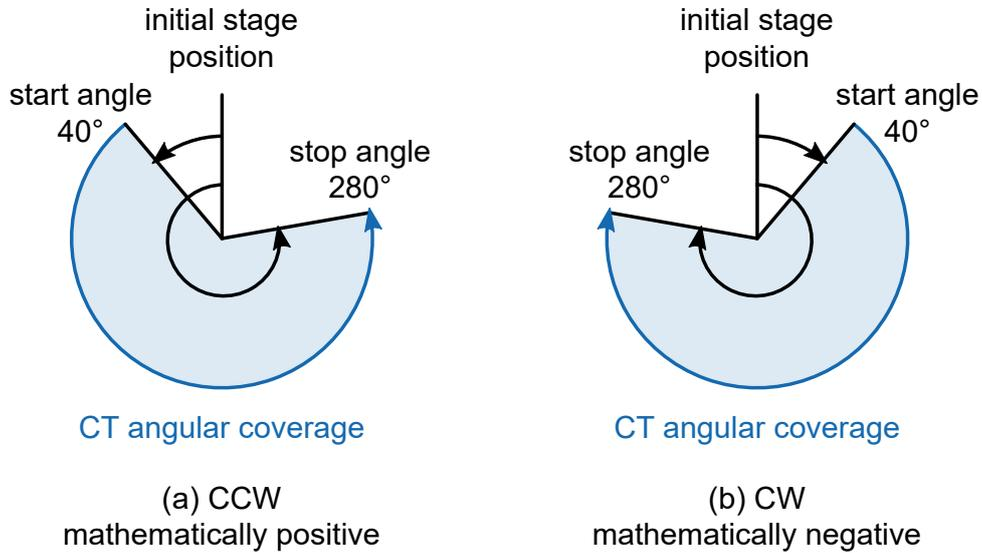
**Fig. 9.1:** The given start angle and stop angle refer to opposite angular positions in **(a)** counter-clockwise or **(b)** clockwise direction (as seen from “above” the stage). They describe the angular range covered by the CT scan.
